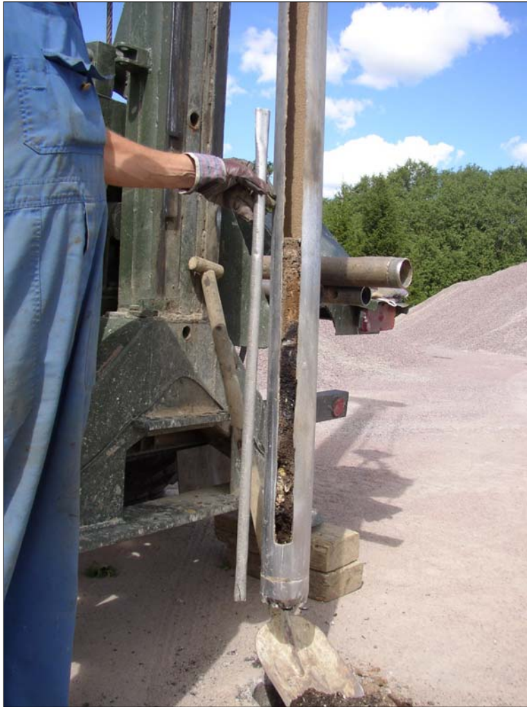
Photo 4026. View to drill core of bore hole 4026; 21.07.2006 Soil is contaminated with shale oil (depth 0,6-1,0 m)
