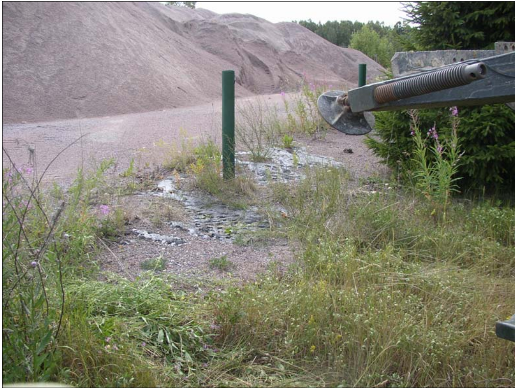
Photo 4000-8. Out flowing hardened shale oil close to bore hole 4025; 21.07.2006
