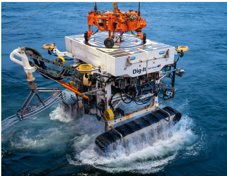
Foto 2. Kaablite paigaldamise seade „Trencher Deep DIG-IT“ (kaugjuhitav). Allikas: https://www.vanoord.com/en/updates/van-oord-completes-cable-installation-crosswinds-hollandse-kust-noord-offshore-wind-park/
