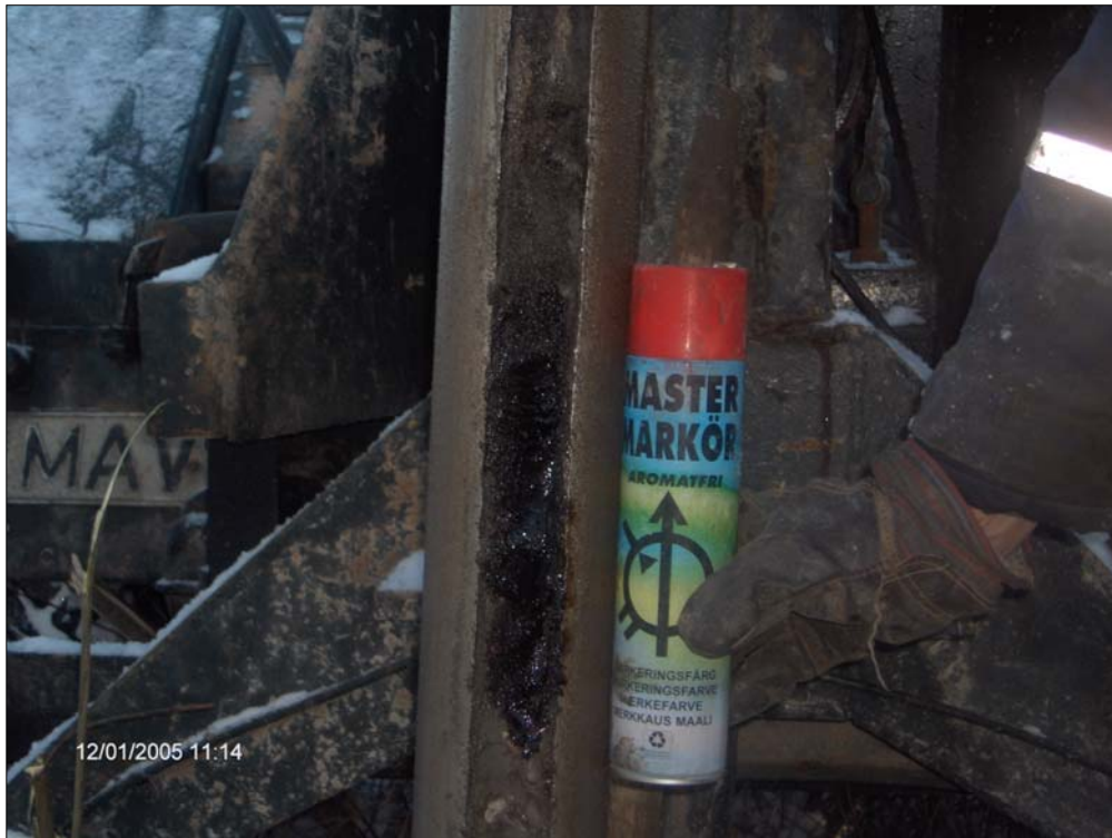
Photo 6519-1. Bore hole 6519 – oily layer between 3,2-3,3 m
