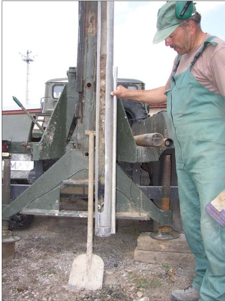
Photo 4700-5 View to the drill core of bore hole 4702; Between 1,6 and 1,8 m black oily layer; photo 12.07.2006
