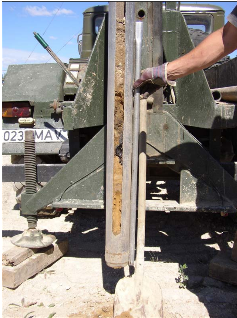
Photo 4509 View to the drill core of bore hole 4509; Between 1,9 and 2,0 m hardened bitumen; photo 17.07.2006
