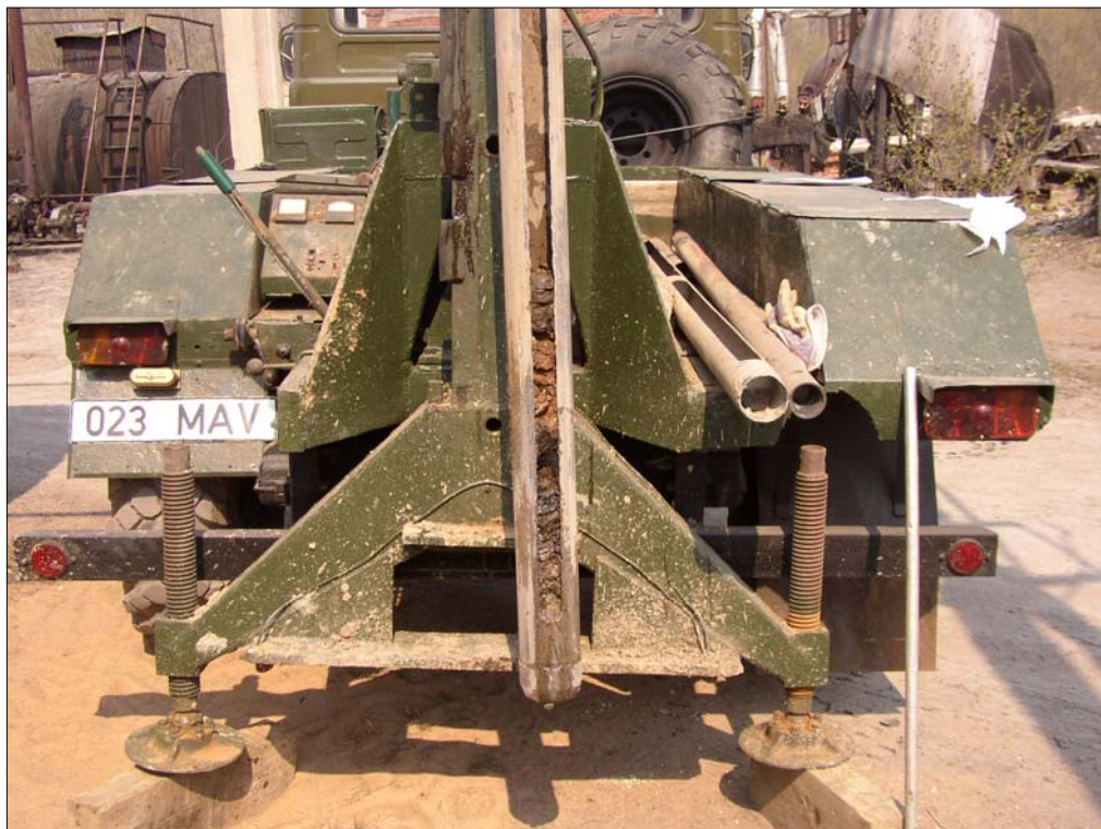
Photo 2508. View to drilling core of bore hole 2508; at depth 0,6 m oily layer
