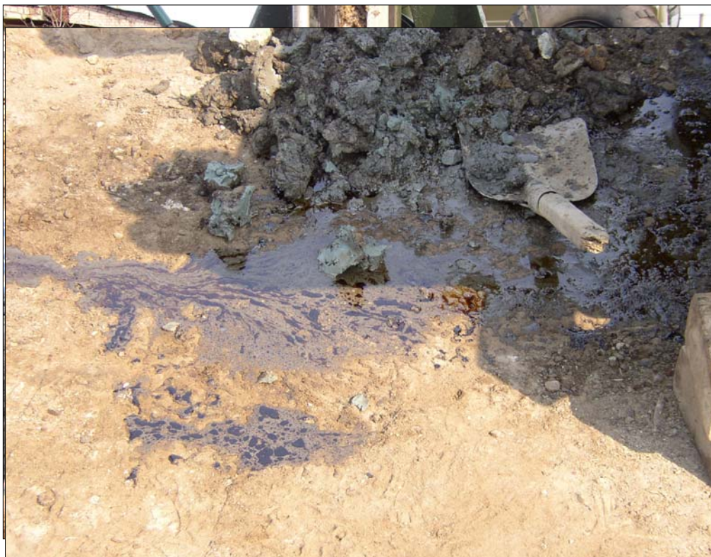
Photo 2416-2. Shale oil from drilling core of bore hole 2416
