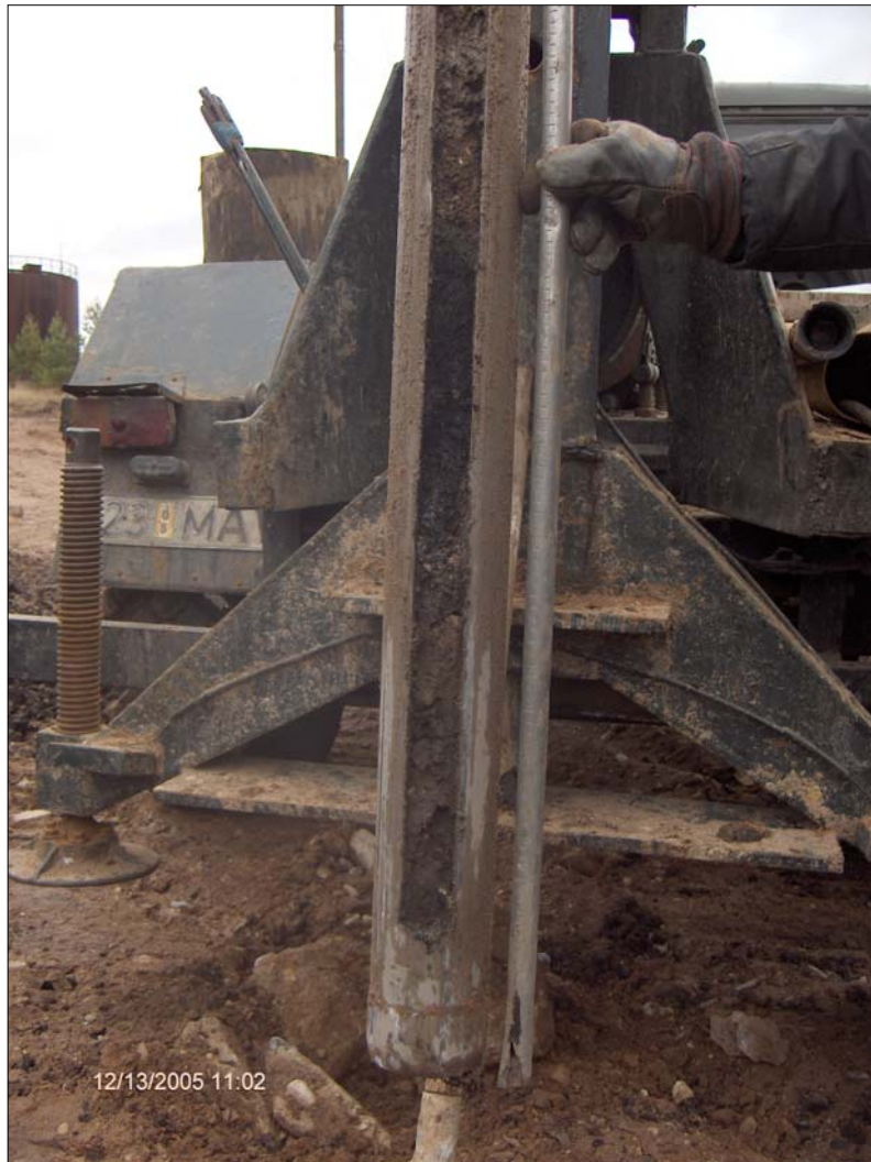
Photo 6925 Hardened oil at depth 2,8-3,2 m in bore hole 6925
