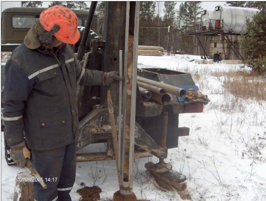
Photo 6917. Drilling core between 2,7-4,1 m in bore hole 6917
