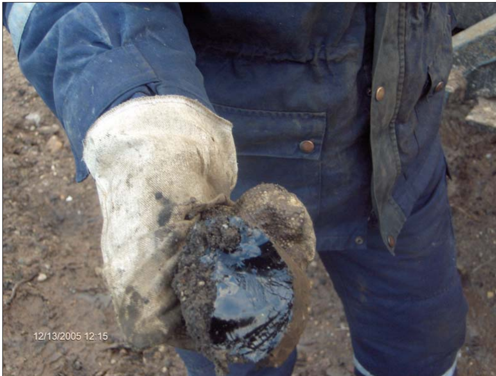
Photo 6927. Hardened oil at depth 1,6-1,7 m in bore hole 6927
