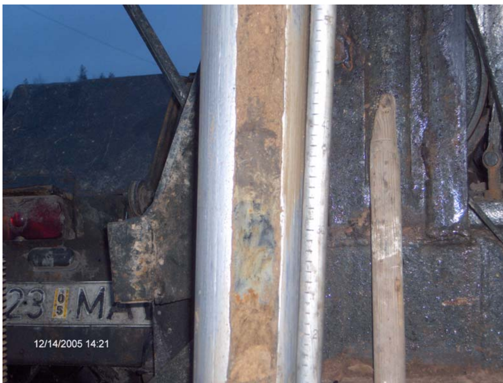
Photo 7301. Black smelling layer in bore hole 7301 at depth at 0,6-0,8 m
