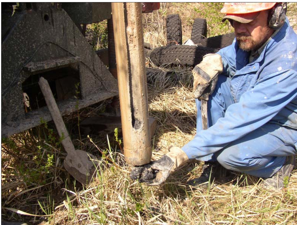
Photo 3407. Hardened oil in drilling core of bore hole 3405 at depth 0,3-0,6 m
