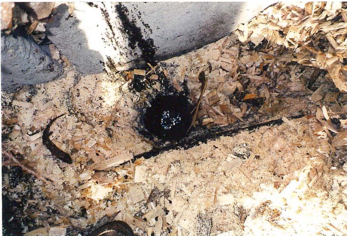
Photo 12. Sampling point PA-4, depth of free phase oil about 0.7 m from ground surface.
