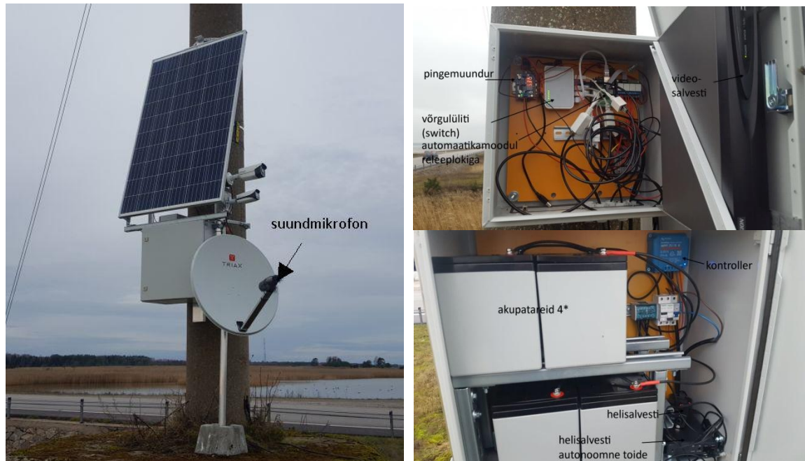
Figure 5. Camera station with audio recording system.
