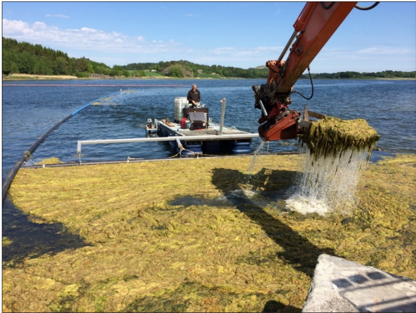
Figure 26. "SLIKKEN" in action, gathering the floating algae mats that have been trapped by booms. An excavator has been used to harvest the green algae to containers on land (photo by G.E. Piene).
