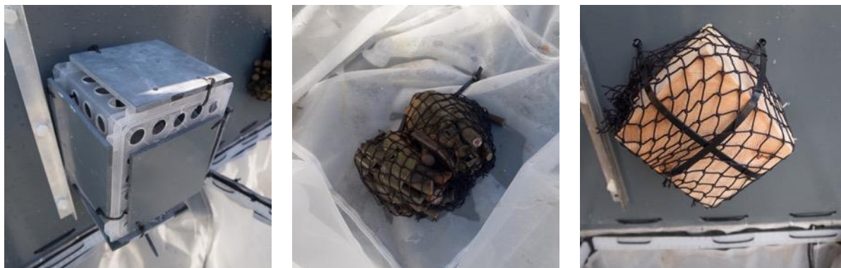
Fig. 3. (Left to right) Inorganic settlement tiles, a kelp parcel and a wood block attached to the lids and bottoms of the lander bins before the lander was deployed (Harbour et al. in press).
