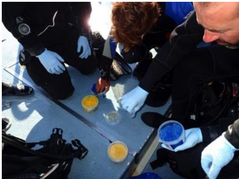
Fig. 3. Preparation of epoxy putty (Photo credits: MedRecover).
